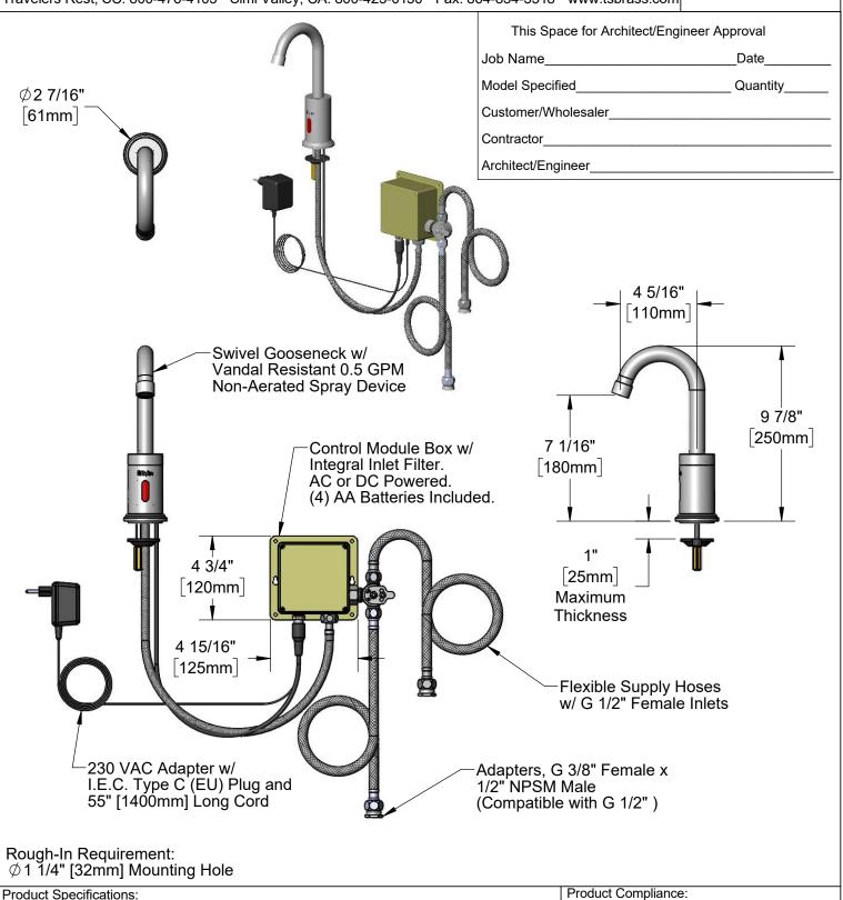
Single Hole Deck Mount Sensor Faucet w/ Swivel Gooseneck, VR 0.5 GPM Non-Aerated Spray Device, Control Module, AC Adapter w/ EU Plug, Mechanical Mixing Valve and Flexible Supply Hoses w/ G 3/8" Female Inlet Adapters
